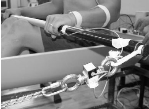
Figure 3: Use of a tensionmeter in a canoe ergometer
