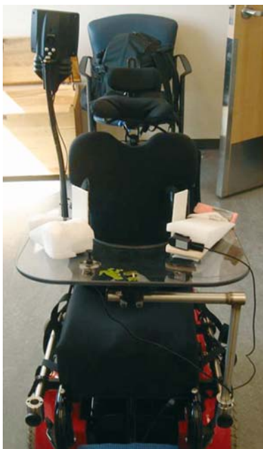
Fig. 6.1. Wheelchair tailor-made for a child with generalised muscle weakness. Note the small switches on the transparent table for the control of the environmental control unit
