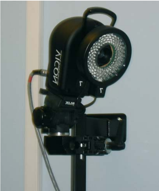
Fig. 8.2. Many gait laboratories utilise 3D gait analysis using the popular Vicon systems
