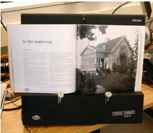
Fig. 12.6. Electric-powered page turner
