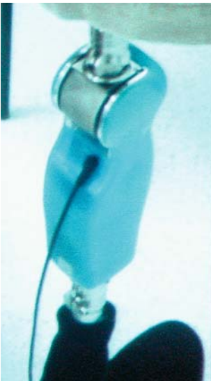
Fig. 10.10. Rheo leg by the company Ossur
