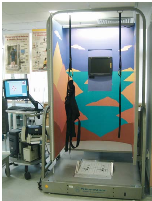
Fig. 19.6. Machine with capabilities for performing the Sensory Organisation Test (SOT)
