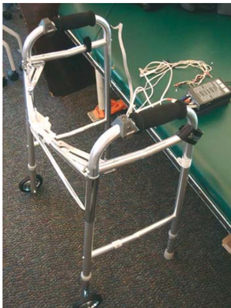
Fig. 12.9. The complete "Parastep" system comes with a walker equipped with control buttons on both sides
