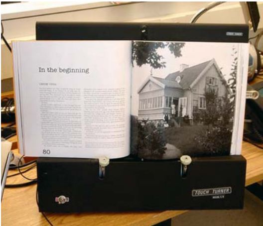
Fig. 6.6. Machine to help the patient to flip over the pages of a book
