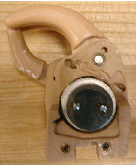
Fig. 10.15. Myoelectric wrist unit for the child amputee
