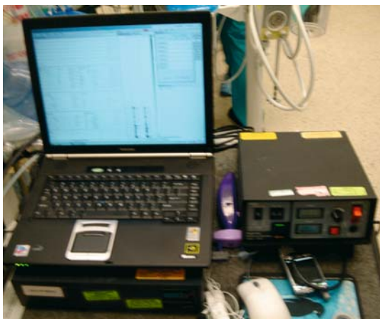
Fig. 7.1. A typical machine used for intra-operative neural monitoring commonly used in spinal operations. Picture shows the commercially used popular Axon System
