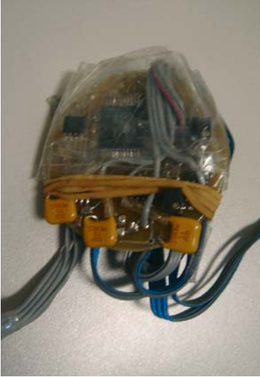
Fig. 6.4. Electronic equipment for mechanomyogram, being used here for a child with a forearm amputation
