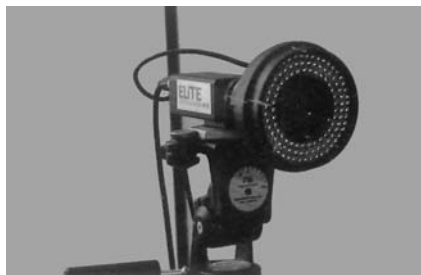
FIGURE 4.21 An IR camera equipped with a stroboscope comprised of LEDs, part of the Italian ELITE system (ELITE, commercial material).
