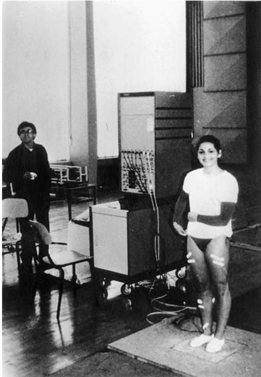
FIGURE 6.17 Female subject with electrodes positioned and fixed, ready to perform the backward somersault from a standing position, take-off from the platform (Biomechanics Laboratory at the Faculty of Physical Education in Zagreb).
