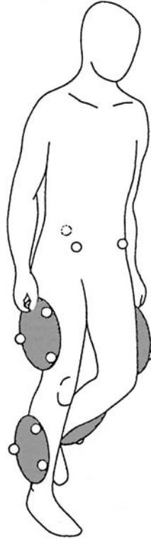
FIGURE 2.2 One possibility for positioning body markers in (clinical) measurements of locomotion kinematics. (From Davis, R.B., De Luca, P.A., and Öunpuu, S. 1995. The Biomedical Engineering Handbook , Bronzino, J.D., Ed., Boca Raton, FL: CRC Press, 381–390. With permission.)
