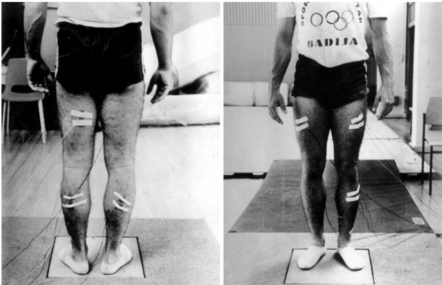
FIGURE 6.8 Positioning of surface EMG electrodes on major lower extremity muscles for kinesiological measurements.
