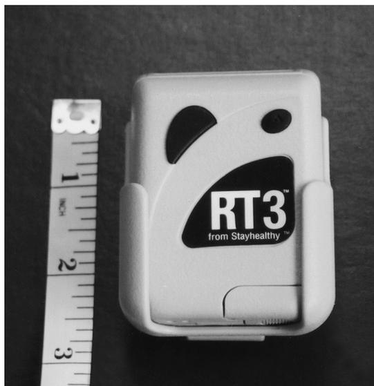
**Figure 6.5** Accelerometer.
