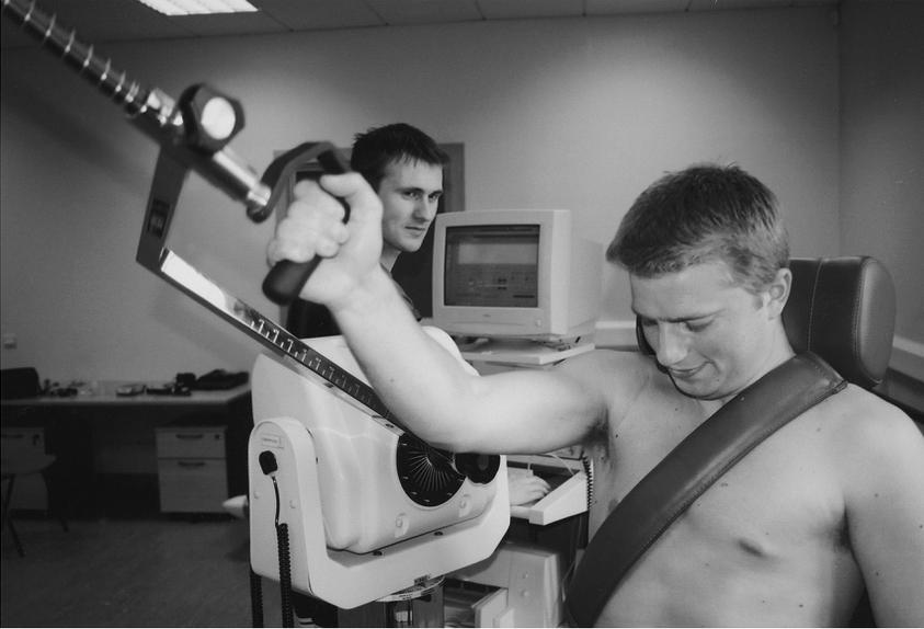
**Figure 6.4** Isokinetic dynamometer to measure muscle strength.
