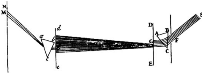
Fig. 2.2 Newton's depiction of the separation of the light spectrum with a prism. Note that the diagram is entirely schematic, with none of the realistic features of Descartes' diagram present
