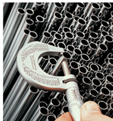
This tool, a micrometer, is used to accurately measure very small distances. Measurements made with it may be recorded in engineering notation.
